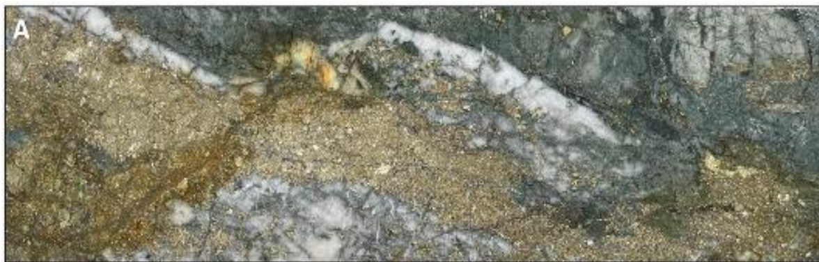
Figure 3. Example of hydrothermal brecciation seen in EB001. Interval at 126.6m depth assayed 6.5g/t Au and 0.47% Cu 4
