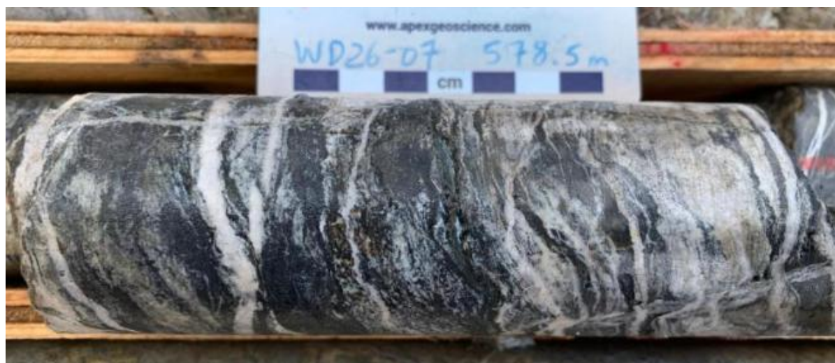
Figure 4: Very strong visual magnetite (black), sphalerite (brownish) and chalcocite (dark grey) bands within exo-skarn in NQ drill core from approximately 578.5m downhole in WD26-07. Laboratory assays for this interval are pending.
