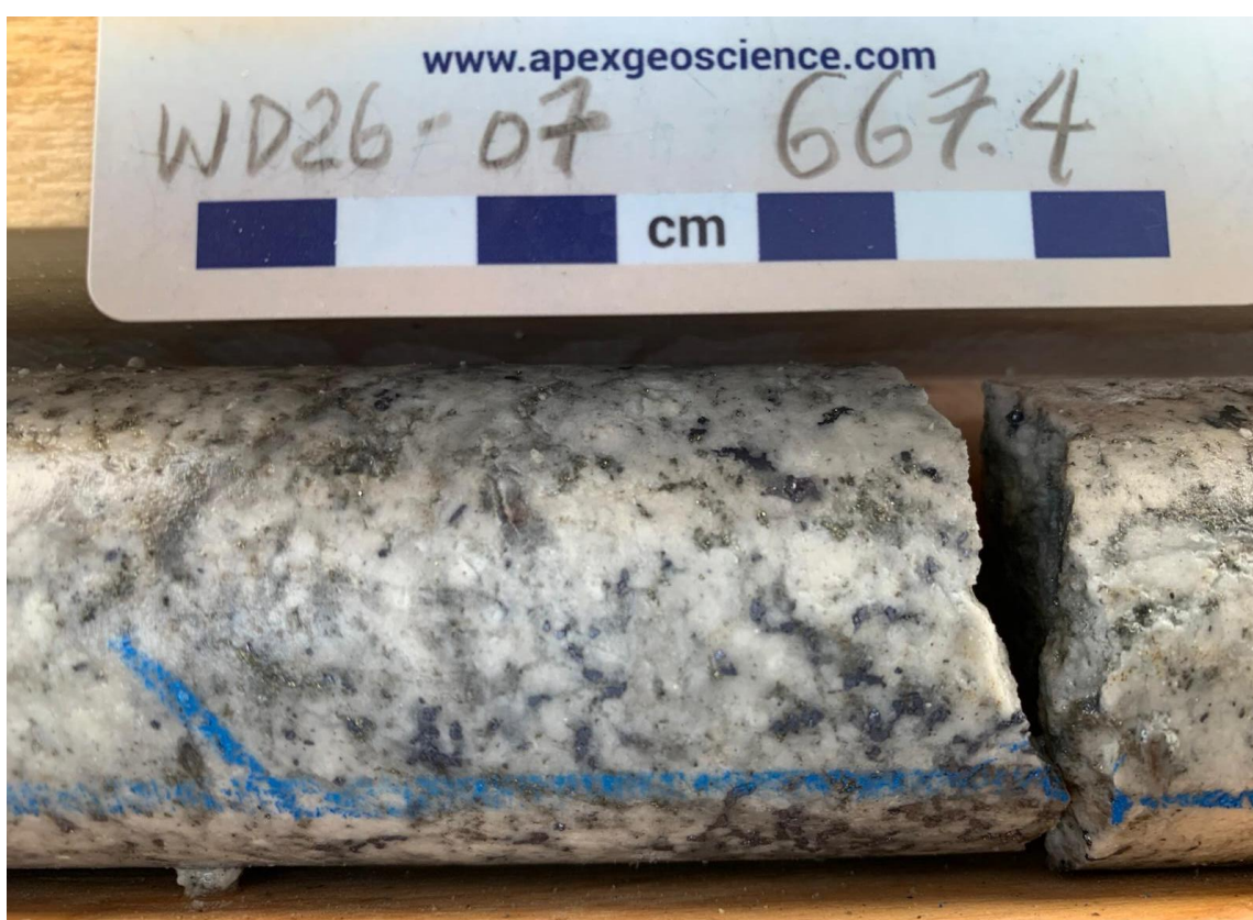
Figure 6: Very coarse disseminated visual molybdenite (blueish-grey) and pyrite (yellowish brass) within altered monzonite porphyry in NQ drill core from approximately 667.4m downhole in drill hole WD26-07. Laboratory assays for this interval are pending.
