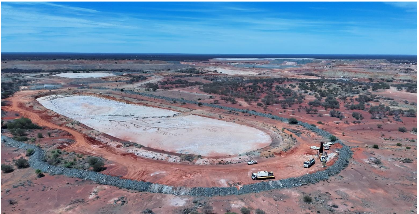
Figure 2: RC drill rig at southern end of Adelaide pit (backfilled with old tailings)
