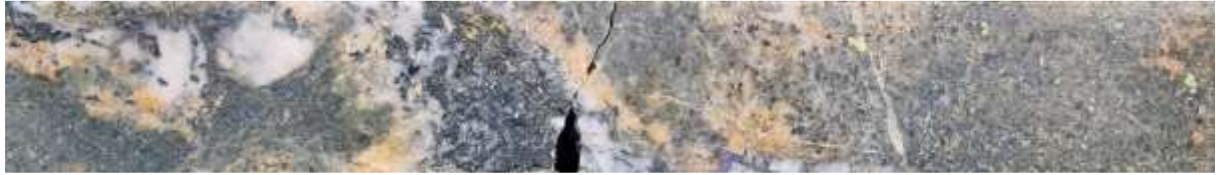
Figure 5: GGDD003 31.85 – 32.15m Quartz-magnetite UST (brecciated) with molybdenite and chalcopyrite. Blebby disseminated chalcopyrite in chlorite-sericite-actinolite-K spar altered crowded porphyry. The associated sample interval 31.1m – 32m returned 0.96% Cu, 0.06g/t Au, 826g/t Mo and 32m – 32.85m returned 0.97% Cu, 0.06g/t Au, 1,365g/t Mo.
