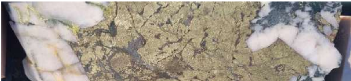
Figure 4: GGDD004 82.30 – 82.50m Brecciated quartz – magnetite UST textures with massive broken chalcopyrite with trace bornite. The associated sample interval 81.87m – 82.81m returned 8.46% Cu, 0.59g/t Au, 25g/t Mo.
