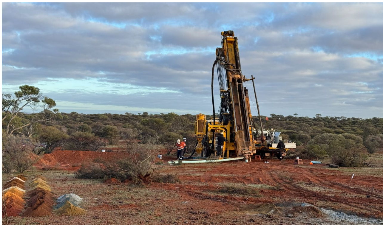
Figure 1: RC Drilling in progress
