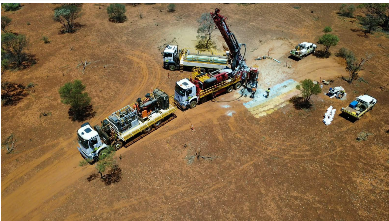
Figure 2 Topdrill's Schramm 685 RC rig drilling the first holes at 140 Foot Well.
