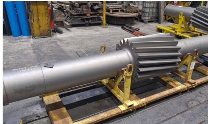
Ball mill pinion ready for shipment
