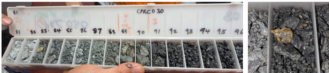
Photo 1 (left): CPRC030 RC chip tray, 81–96m. Photo 2 (right): RC drill chips from sample NM49773 (82–83m) showing visible gold.
