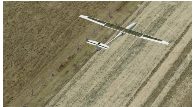
Halocell perovskite solar arrays fitted along the wings (left); Pegasus over the Queensland test range (right)
