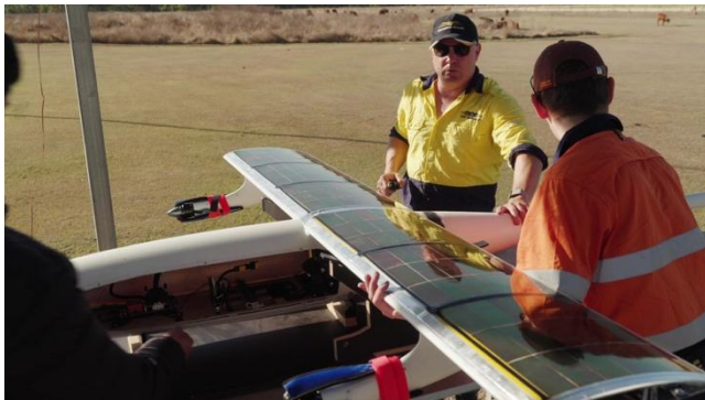
Halocell perovskite solar arrays fitted along the wings (left); Pegasus over the Queensland test range (right)
