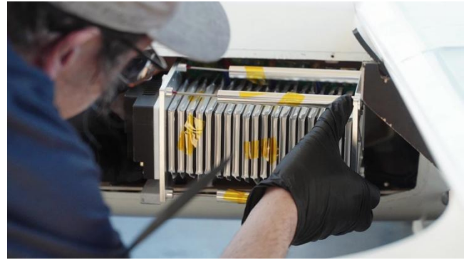
Pegasus on its launch ramp prior to take off (left); the Li-S Energy battery pack being installed in the Pegasus fuselage (right)
