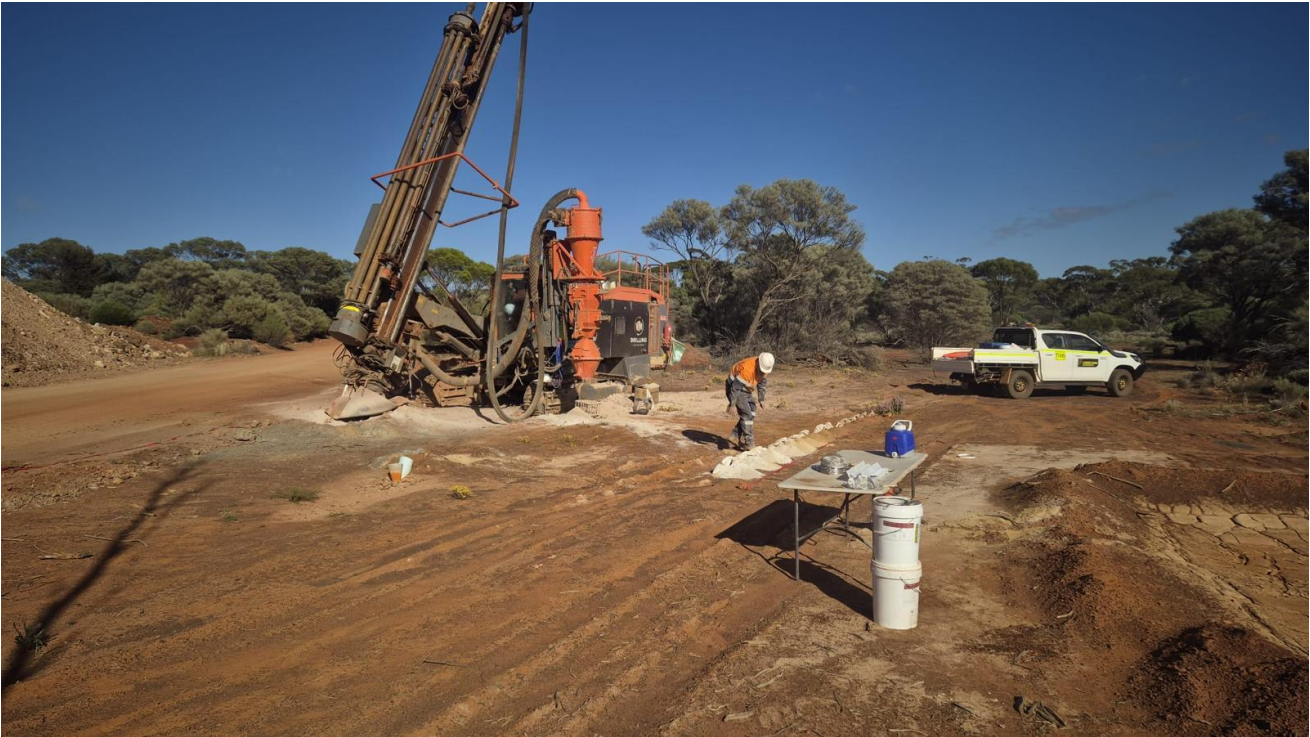
Figure 9: Grade Control Drilling – Johnson Range
