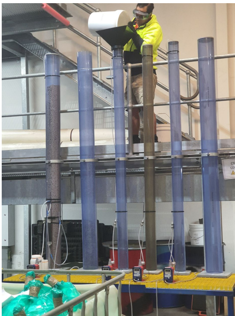
Plate 2 – Loading of variability column leach tests with Apollo Hill agglomerated ore material types – early July 2026
