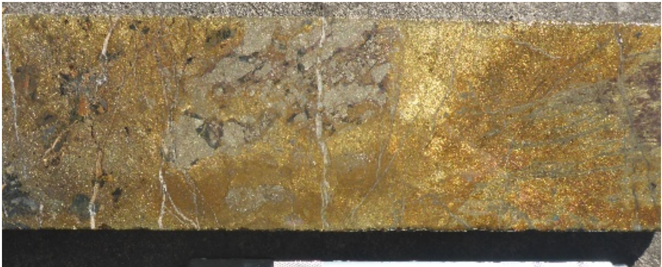
Figure 4: DTD002: 481.2m 60cm interval of massive chalcopyrite + pyrite + minor bornite, in quartz magnetite brecciated vein – sample assayed 25.6% Cu & 1.29g/t Au.
