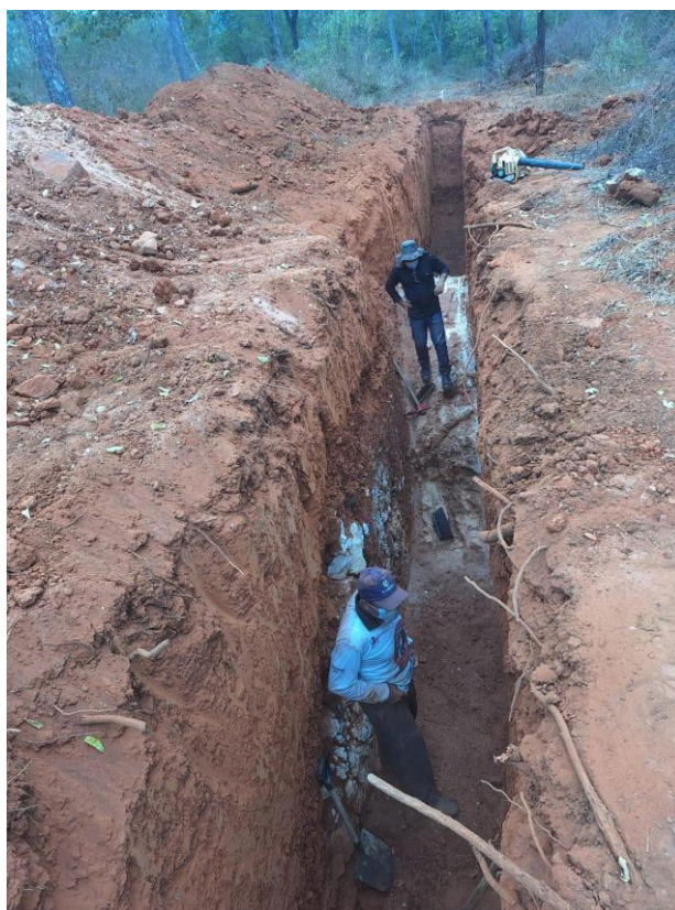
Figure 7: Channel sampling undertaken earlier in 2026 at Trench TR01, with exposed pegmatite shown towards the rear of the trench at the Mauricio Target.
