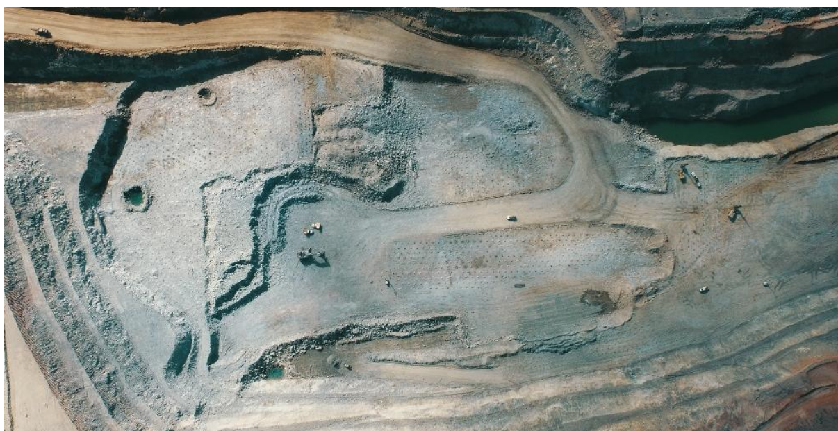
Plate 4: Completed drill and blast patterns in Devon pit (Photo taken 15 July)
