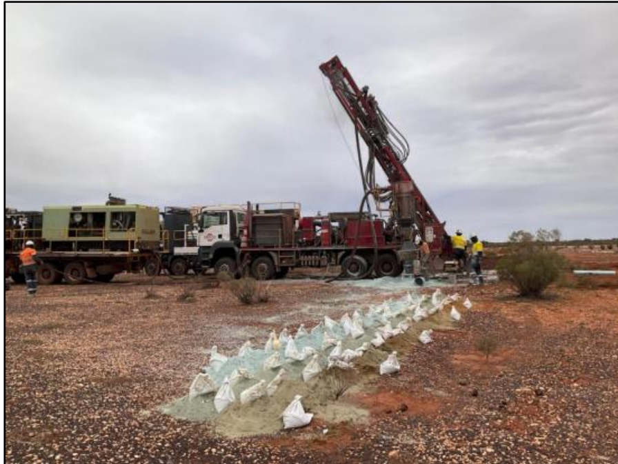
Figure 1: RC Drilling rig at Beatty Park Sth
