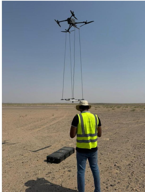
Figure 3 UAV Magnetic Survey at Sukhaybarat South
