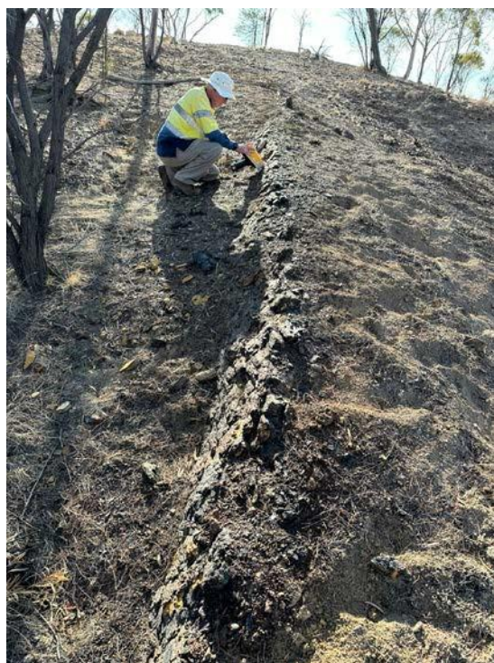
Base Metal Target - Outcropping fine-grained sedimentary rock of the Ronlow Beds with cleavage steeply dipping toward NE - strike NW-SE - yellow-ochre, black & brown limonite possibly derived oxidation of sulphides at depth. The petrology sample collected at this location (GDA2020 343440mE and 7483340mN Zone 55) and shown in Figure 11.
