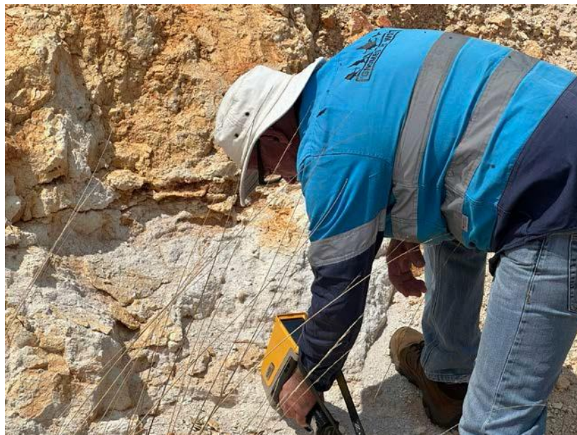
REE Target - pXRF sampling of white weathered kaolinitic fine-grained sediments adjacent to the prominent scarp
