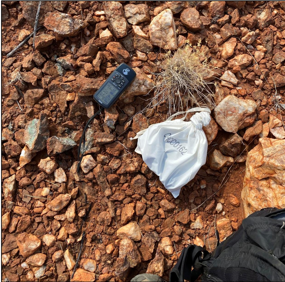
Figure 3 Malachite-bearing outcrop associated with ultramafic-mafic dyke from the Coondina project.
