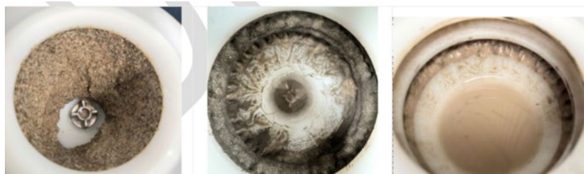
Figure 7: Three-stage Falcon gravity concentrates.
