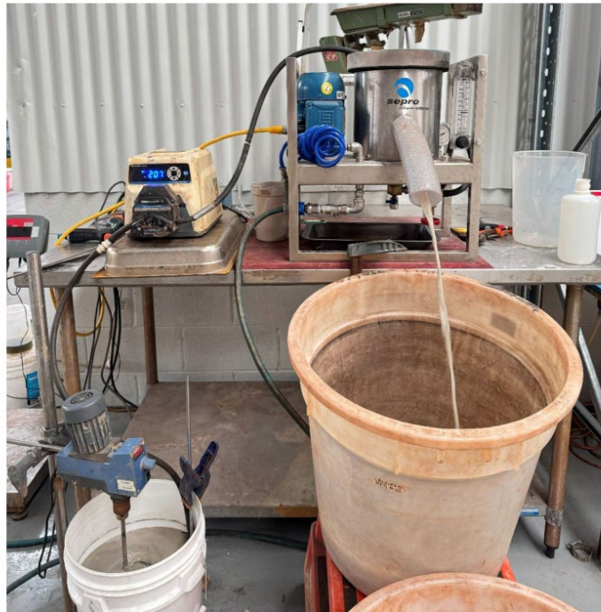
Figure 6: Falcon gravity separation test setup.
