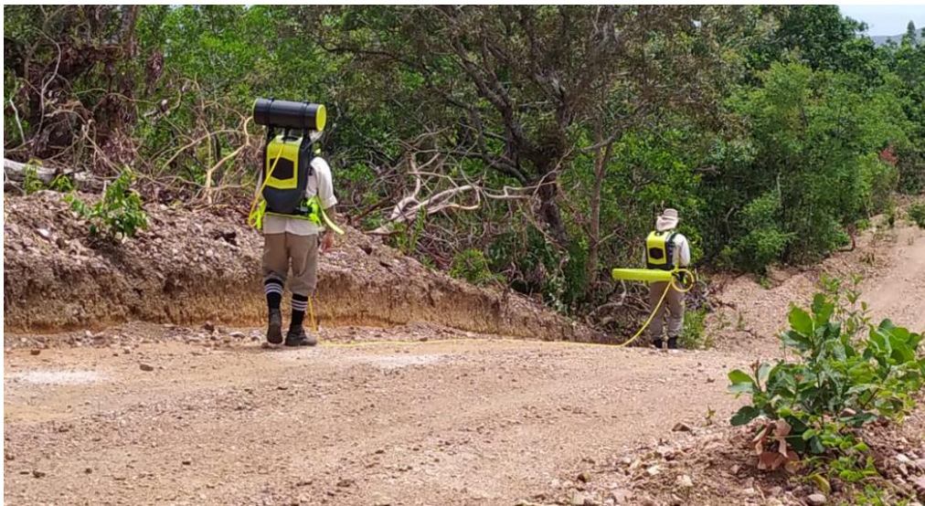
Figure 3: Loupe portable electromagnetic survey underway at Bluebush.
