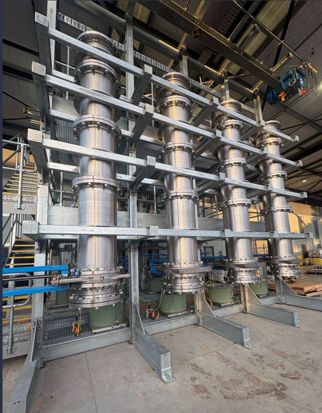
4m high pilot-scale leach columns
