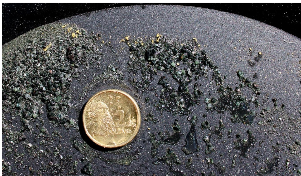
Figure 1: Visible gold panned from 26HHRC179 (91-92m), with 20mm coin for scale. 4
