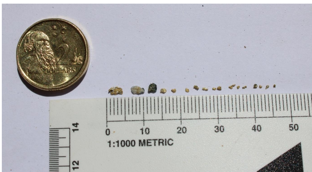
Figure 2: Close-up image of gold panned from 26HHRC179 (91-92m), with coin and ruler for scale. 4
