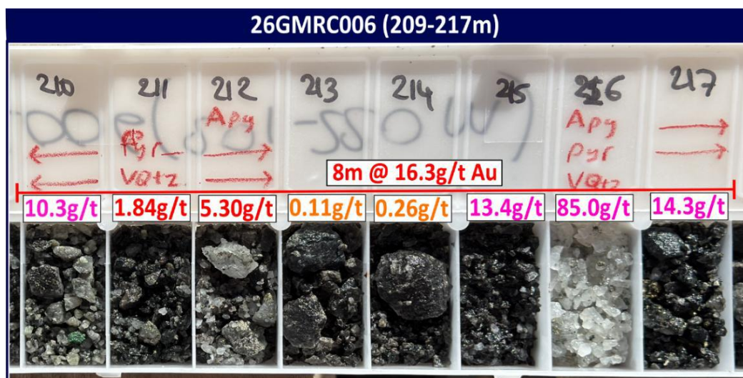
Figure 12: RC chip tray of hole 26GMRC006 (209m - 217m downhole) showing broad intersection of 8m @ 16.3 g/t Au with individual gold grades (to 85.0 g/t Au) shown underneath.
