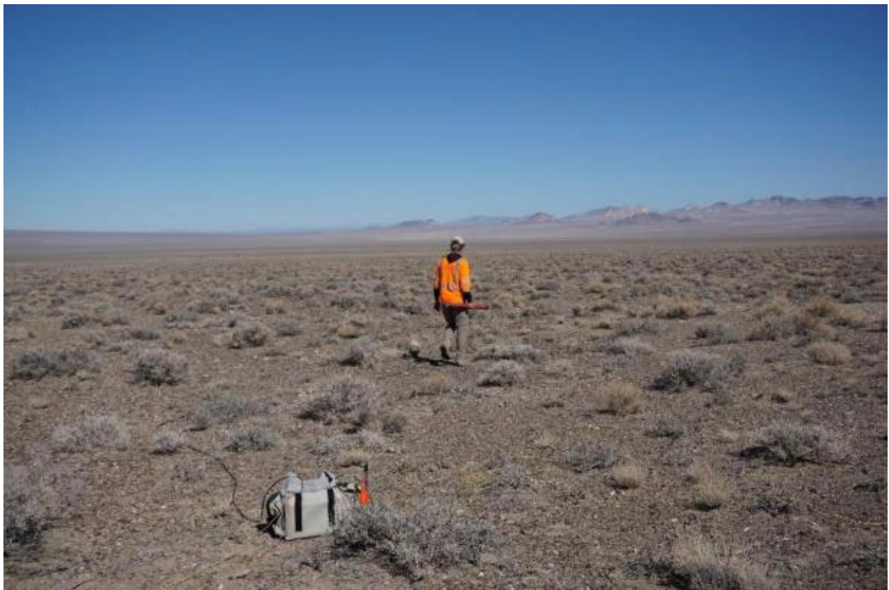
Figure 6. CSAMT SURVEY RECEIVER DEPLOYMENT AT THE ALKALI FLATS PROJECT
