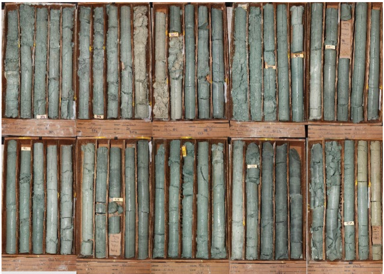
Figure 9. CORE OF SEIBERT FORMATION CLAYSTONE (AF3-CO2, 330ft - 440ft)
