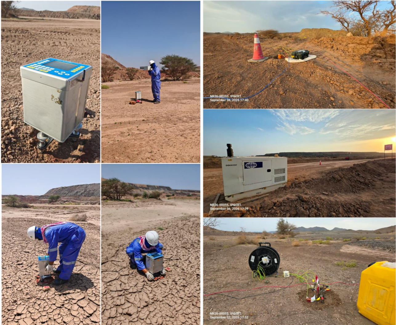
Figure 25 – Orientation geophysical surveys - Gravity & ERT
