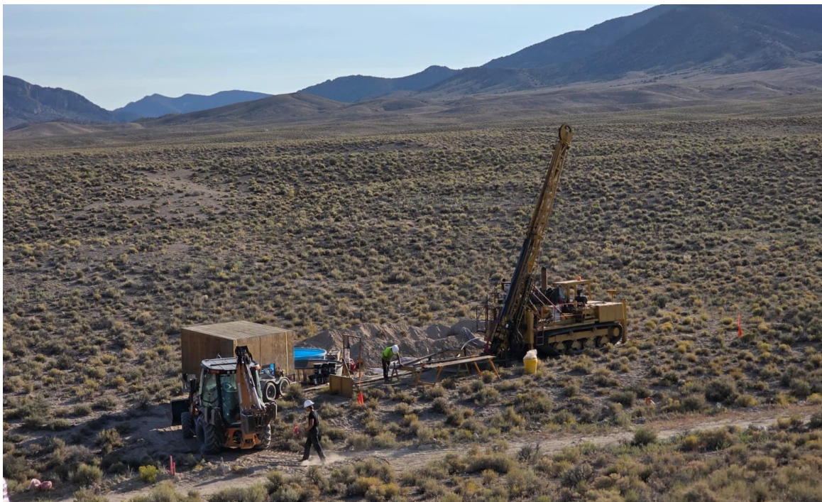
Figure 3. Diamond drill rig set up over drill-hole RMDD009 (Plan ID RMP006).
