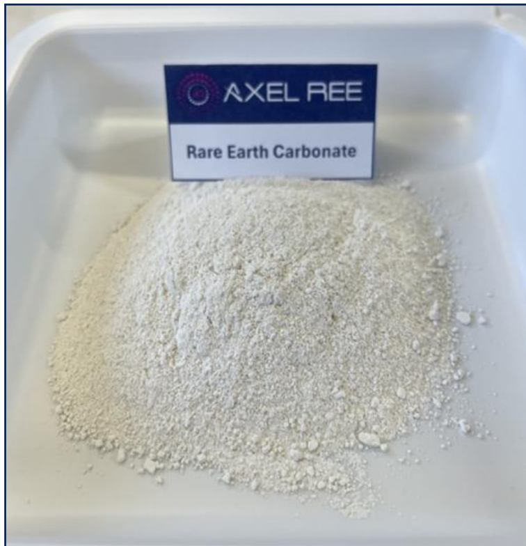
Image: Axel's first mixed rare earth carbonate derived from its in situ recovery column leach tests from the Woolrich ionic adsorption clay deposit.
