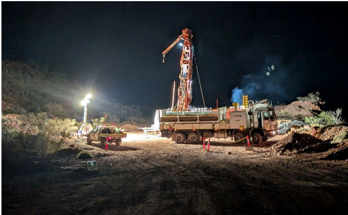
Figure 3: Phase 1 diamond drill rig on pad at Mons Cupri, Whim Creek Project, Pilbara WA
