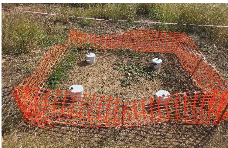
Figure 3: Example test cell with static chambers in situ at the NBRC landfill site
