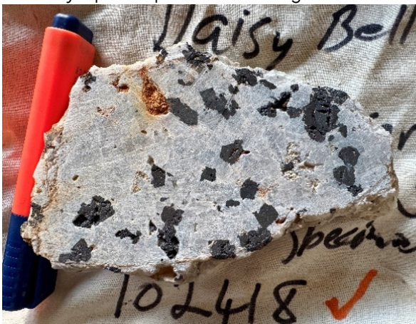
Figure 5a. A photo of rock chip SampNo 102418 collected from a wolframite-bearing greisen outcropping near the top of Billings Knob in the historic Daisy Bell mine and assaying 0.14% W. Figure 5b. Historic stockpile ore remaining at Daisy Bell. Visual observations of mineralisation are qualitative only and should not be considered a proxy for laboratory assay results or an indication of grade. The reported grades for samples shown are based on laboratory analysis.
