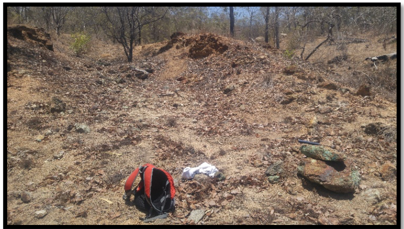
Figure 4a. Rock chip sample 102248 (13.3% Cu and 11.5% Bi, see Table 1) was collected from the top boulder in the bottom right of the photo within historic excavations at Muirson Pinnacle. Figure 4b. A close up of the retained sawn half of sample 102248 showing copper oxide mineralisation. Visual observations of mineralisation are qualitative only and should not be considered a proxy for laboratory assay results or an indication of grade. The reported grades for samples shown are based on laboratory analysis.
