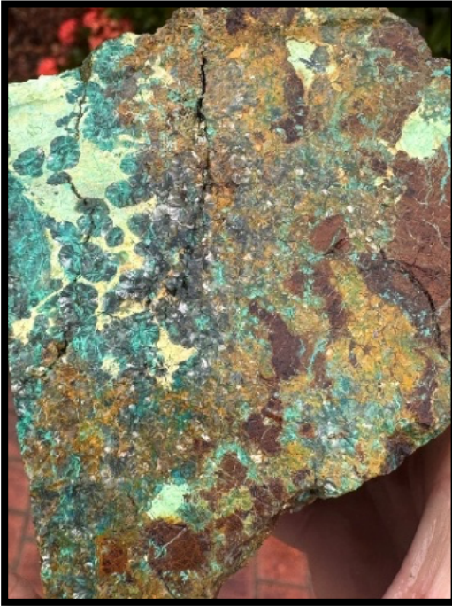
Figure 4a. Rock chip sample 102248 (13.3% Cu and 11.5% Bi, see Table 1) was collected from the top boulder in the bottom right of the photo within historic excavations at Muirson Pinnacle. Figure 4b. A close up of the retained sawn half of sample 102248 showing copper oxide mineralisation. Visual observations of mineralisation are qualitative only and should not be considered a proxy for laboratory assay results or an indication of grade. The reported grades for samples shown are based on laboratory analysis.
