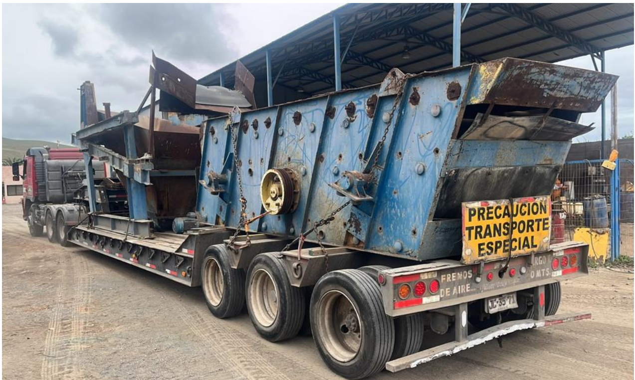
Image 3: Three-deck screen for refurbishment being delivered to Islon earlier this week
