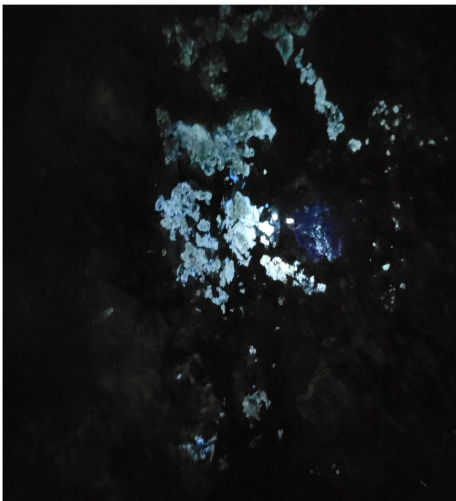
Figure 8: Exposure on the 400-foot level photographed under short-wave ultraviolet light, showing scheelite fluorescence.
