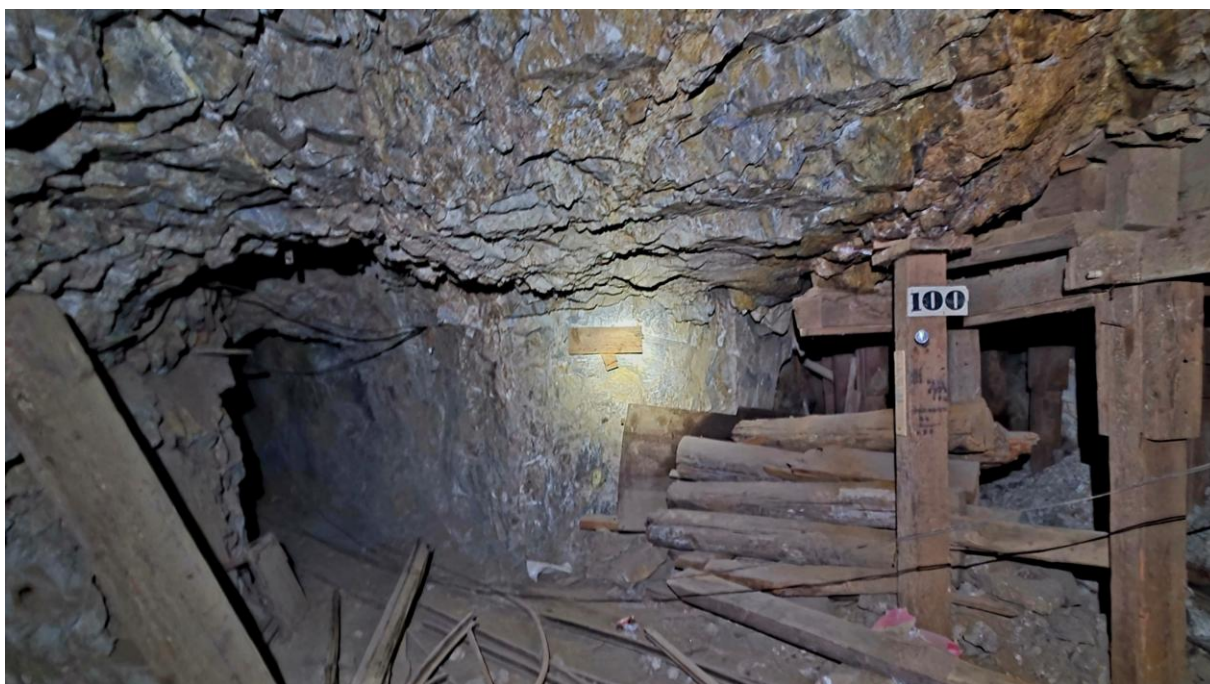
Figure 5: 100L at the Main Shaft looking ~northeast. Red-brown garnet skarn is situated above the 100 level sign.
