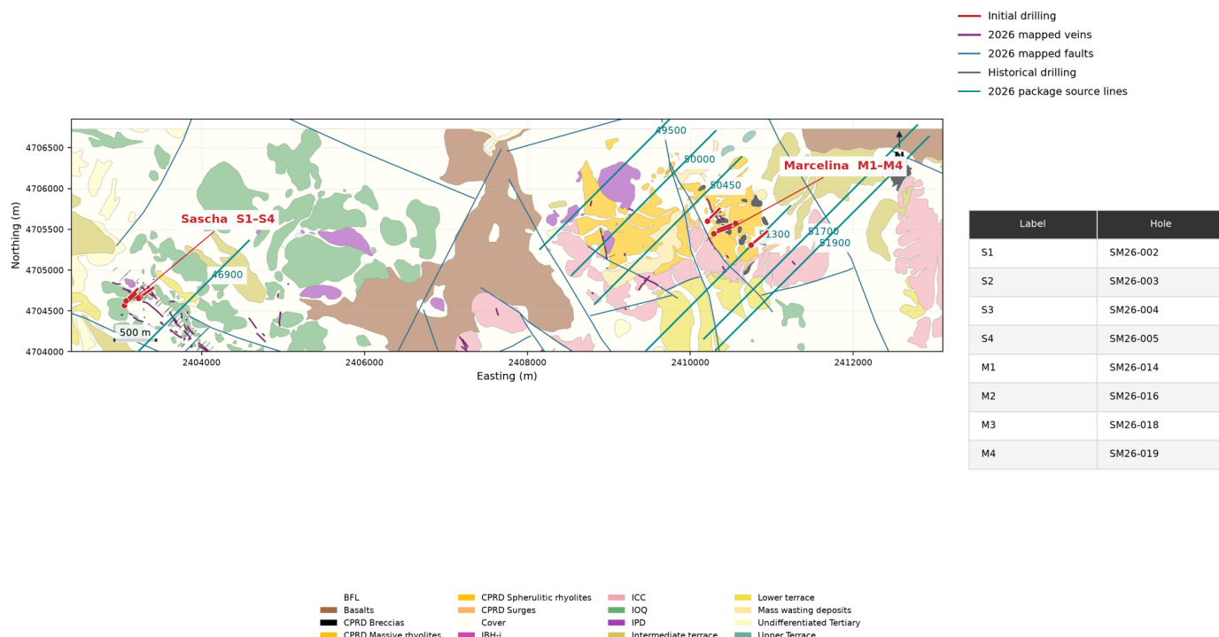
Figure 1 – Sascha Marcelina Project geology showing 2026 IP survey lines, 2026 mapped veins and faults, historical drilling and the initial drill holes at Sascha (S1 to S4) and Marcelina (M1 to M4).
