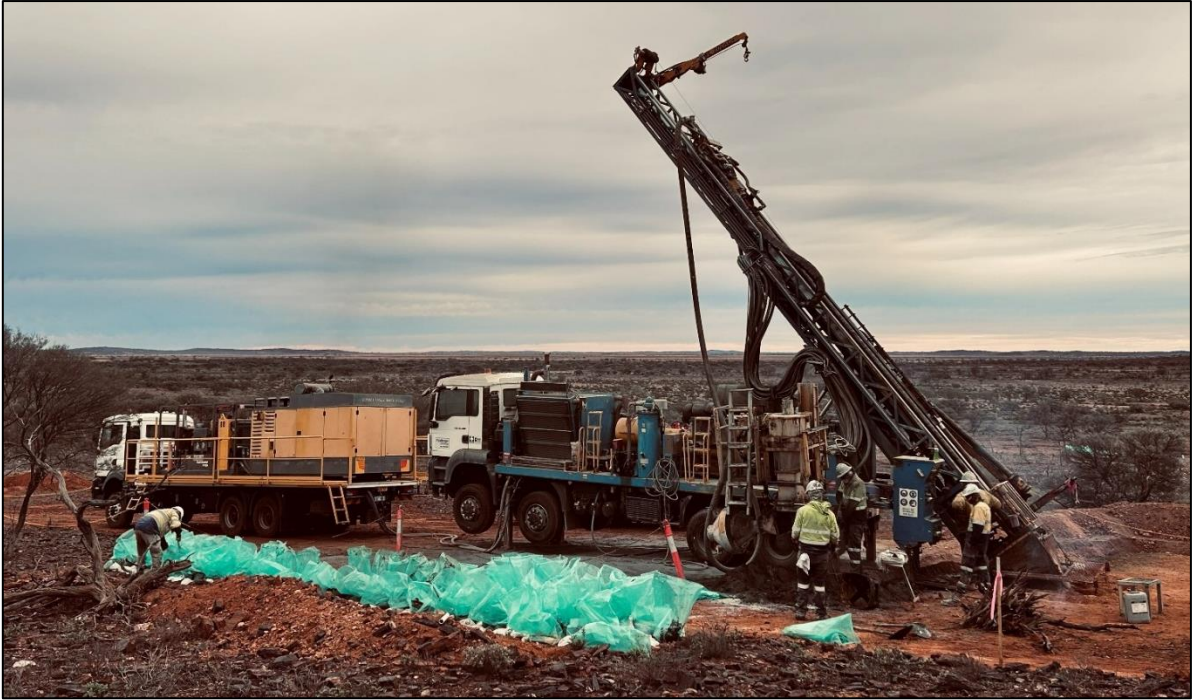
Figure 1. RC drilling at the Austin Gold Project during the September 2026 quarter.
