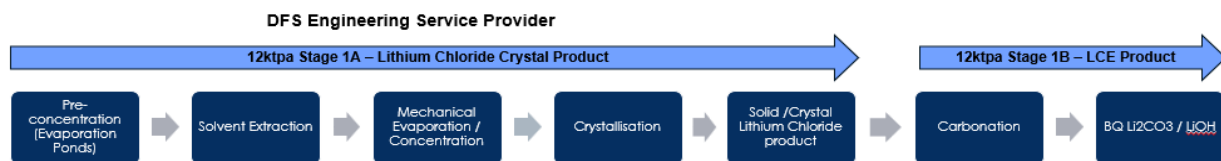
Figure 1. Rincon Lithium Project – Process Flowsheet
