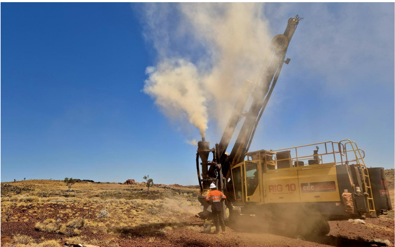
Figure 1: RC drill rig at the Gingarrigan Prospect, Woodie Woodie North Manganese Project.
