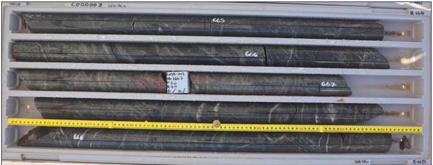
Figure 2: Core tray photo from Coogee West Diamond Hole C000002 664.6m – 668.8m down hole highlighting one of the dolerite units intersected showing brittle deformation with chlorite-epidote-K feldspar alteration and quartz-carbonate veining
