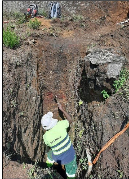
Figure 6 and 6A: Field staff inspect and sample laterite in Sulima West Trenches
