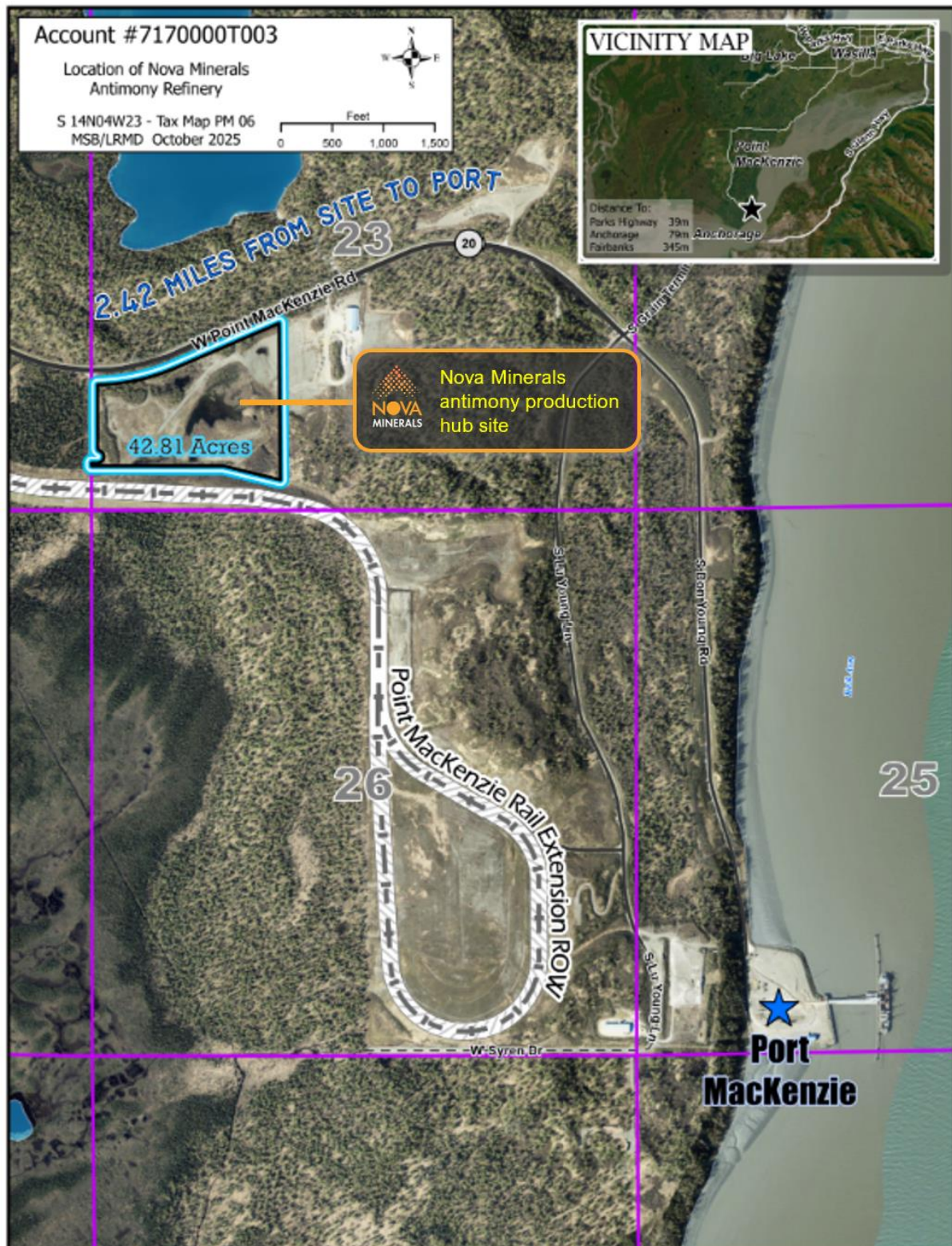
Figure 1. The Port MacKenzie Rail Extension will link directly to Nova Minerals' antimony refinery site and include a rail siding on site
