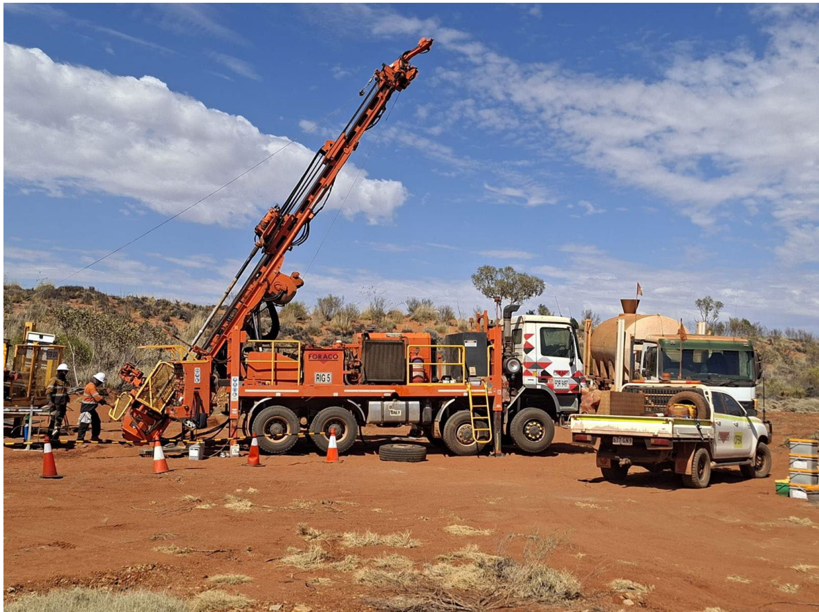
Image 1 – Diamond Drill Rig Onsite
