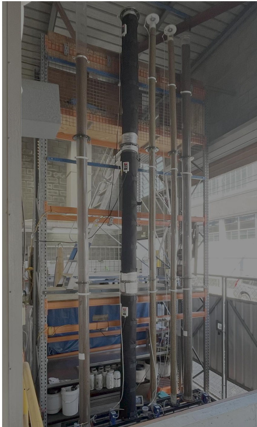
Figure 1 Sybella Kary Zone: Large-diameter six-metre column leach tests in progress on -20mm crushed Saprock and Transitional ore.
