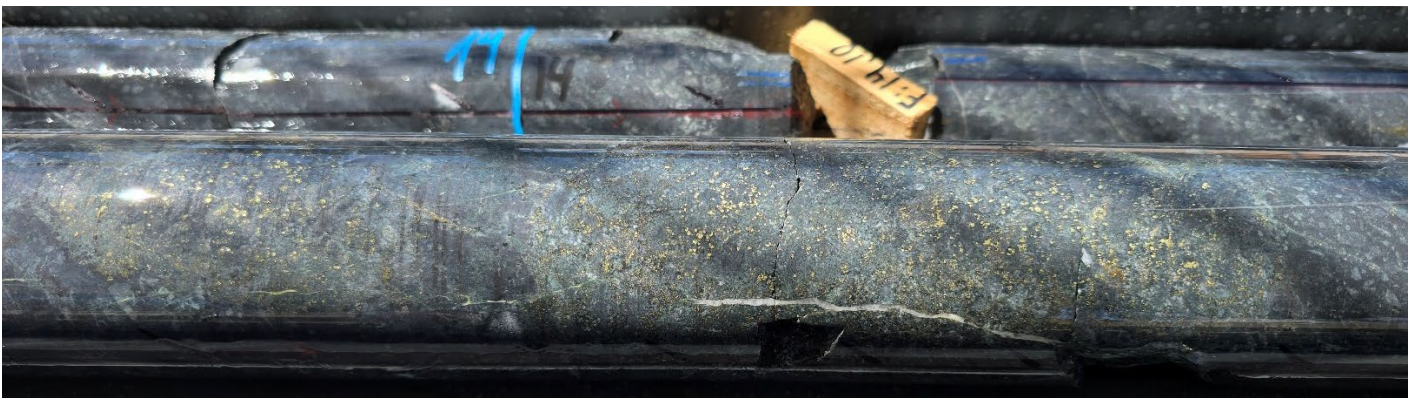
Photo 1. Heavy disseminated chalcopyrite from 13.0–13.4m, LLD0001.
