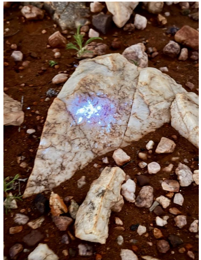
Figure 2: Photo of scheelite fluorescing under short wave ultraviolet light within quartz subcrop and float at Nina. Near historical sample 9925 (7335841N, 389769E) which returned 0.7% WO 3 .
