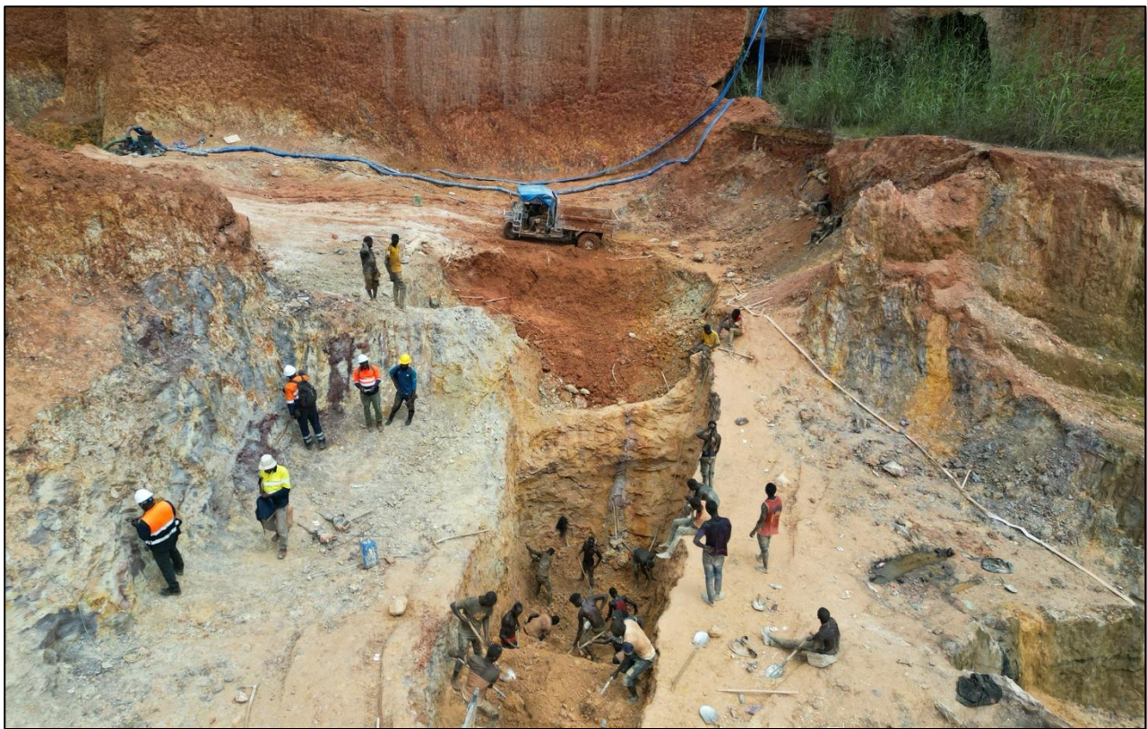
Figure 2 - Sampling underway at the southern Malikila Prospect, assessing gold distribution within an interpreted dyke, along its contacts and in adjacent altered host rocks.
