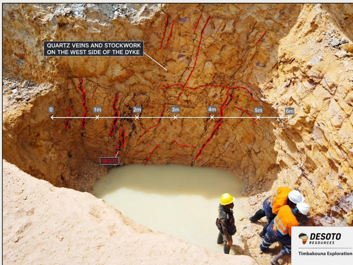
Figure 1 - Quartz veins and stockwork exposed in weathered host rocks on the western side of the interpreted dyke at the southern Malikila artisanal pit, Timbakouna. Red dashed lines highlight vein traces, with a structural measurement of 080°/70° annotated. The approximately 6m marked traverse indicates exposure length, not a confirmed mineralised width.
