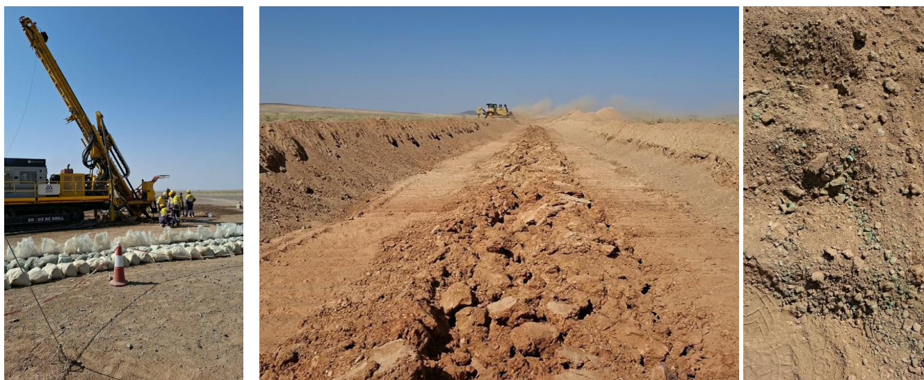
Figure 2. RC drilling and trench excavation at As Safra during the Phase 2 program.
