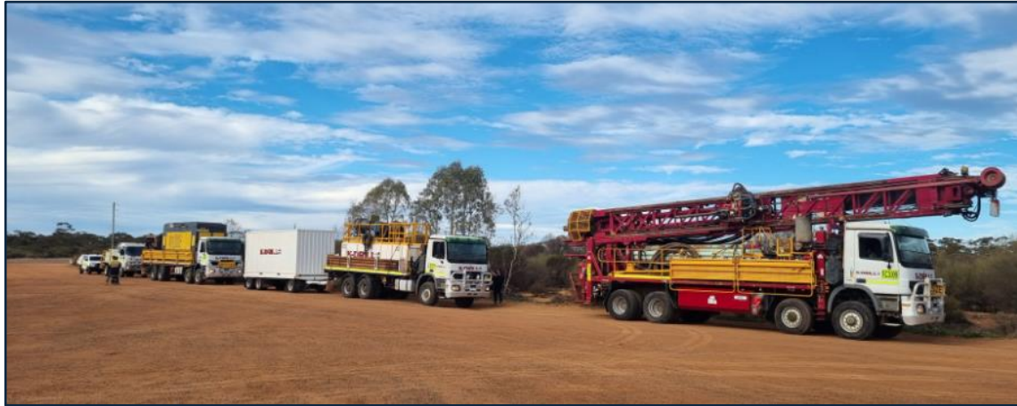
Figure 2: K-Drill RC rig to commence drilling at New Waverley.
