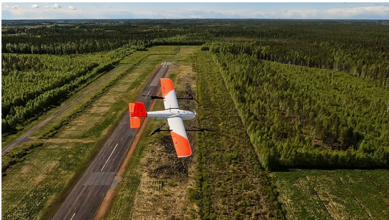
△ Figure 2 Radai drone used to collect high-resolution magnetic and radiometric data
