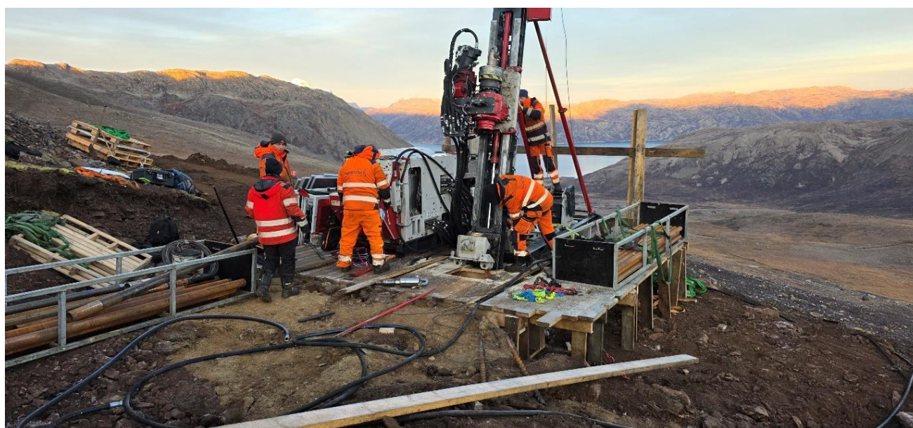
Figure 1: Diamond drilling underway at Grønnedal during the October 2026 field campaign
