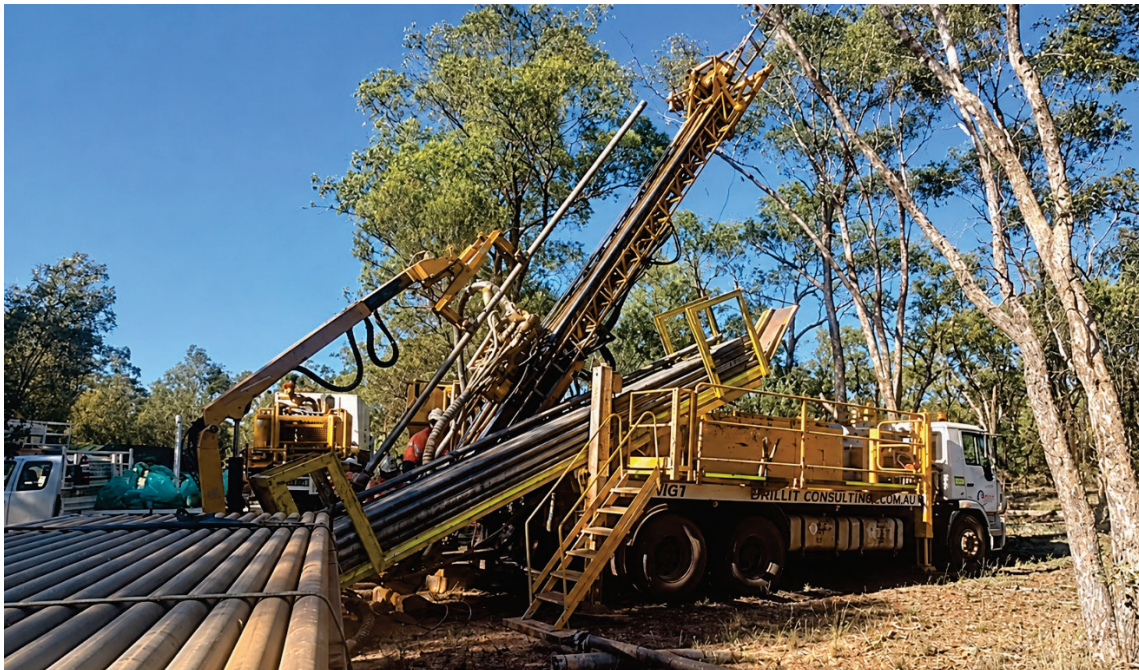
Photo 1: Reverse Circulation drilling rig operating at the Wilga Flats Project
