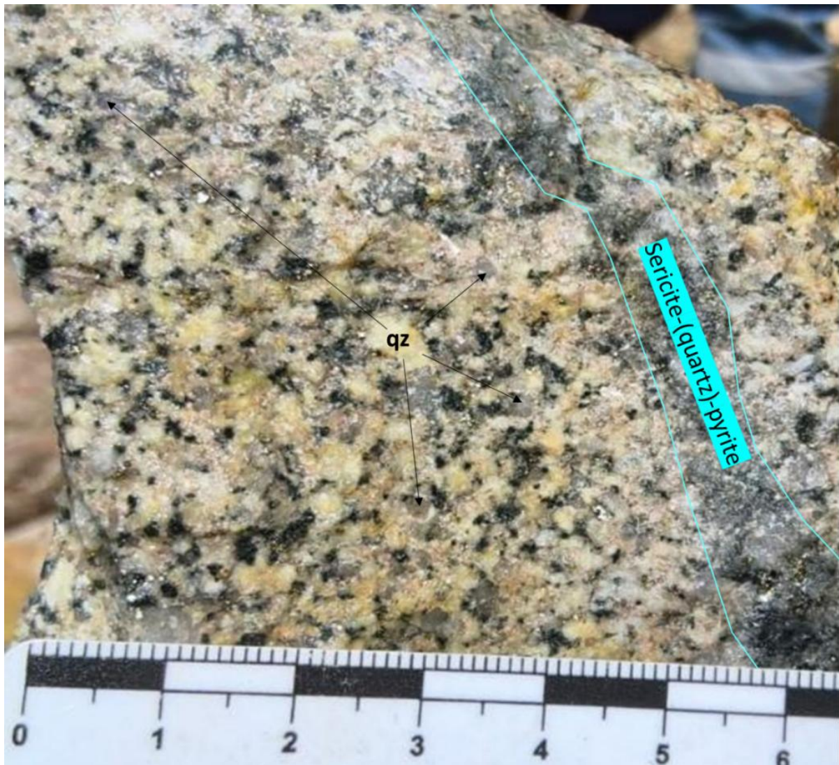
Figure 4: Altered granodiorite cut by quartz-sericite-pyrite veinlets within target zone 2. The observed alteration and veining provide further surface evidence of hydrothermal activity associated with the broader Cu-Mo system and support upcoming drilling to test the mineralised system at depth. Sample 000014 returned 0.43% Cu, 0.038% Mo and 3.2 g/t Ag.
