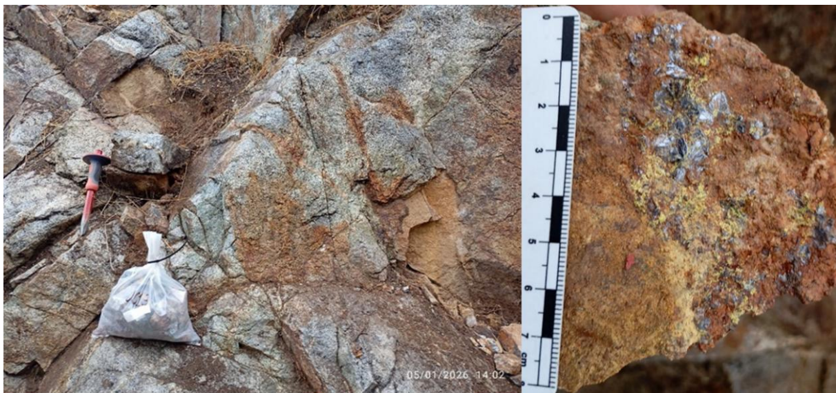
Figure 6: Outcrop of sample 000013: moderate quartz-chlorite-limonite-pyrite-chalcopyrite-molybdenite-Cu oxides fracturing in chlorite altered granodiorite (a fracture detail on the right side) reported 0.19% Cu, 6,270 ppm Mo, 4.2 g/t Ag. Located within target zone 2 with coordinates E: 222,887 mE N: 8,847,024 mN.
