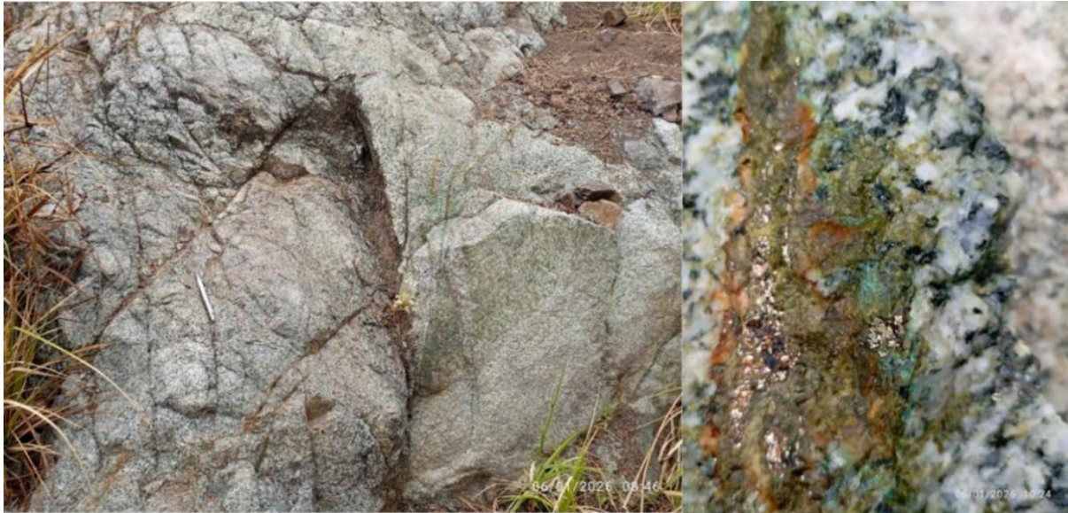
Figure 5: 2 x 2 m outcrop of chlorite-altered granodiorite with moderate chlorite-pyrite-chalcopyrite-Cu oxides veining (see detail of vein at right) – sample 000014 reported 0.43% Cu, 380 ppm Mo, 3.2 g/t Ag. Located within target zone 2 with coordinates E: 222,885 mE N: 8,847,018 mN. In the same area, a selective sample of quartz-pyrite-chalcopyrite-Cu oxide veining cutting chlorite altered granodiorite (sample 000011) reported 0.49% Cu, 419 ppm Mo and 2.1 g/t Ag. Located within target zone 2 with coordinates E: 222,867 mE N: 8,846,964 mN.
