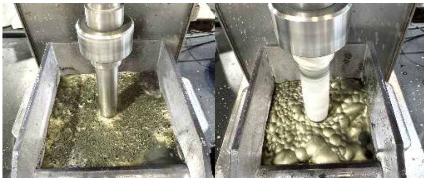
Figure 4: Photo of Flotation tests for WND2 (Wallace North), rougher stage (left) and cleaner stage (right)
