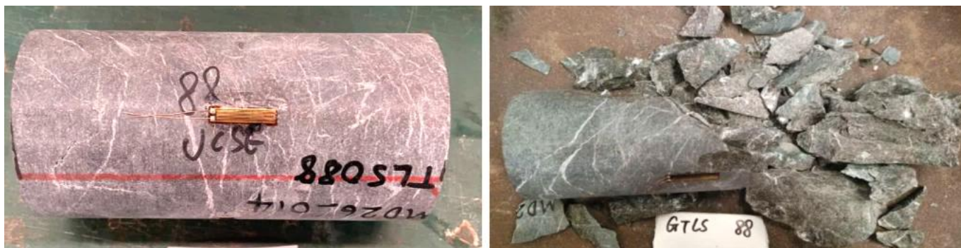
Figure 6: Photos of sample GTLS088 (GAM pit), before and after UCS & Deformation testing.
